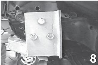
Once the middle braces are bolted to the frame, drill the 3/8" holes for each side. Use the 3/8"-16 x 1 1/4" hex bolt, 3/8" lock washer, and 3/8 flat washer.
