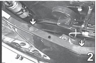
2. Remove the Phillips screws from the top of the plastic fascia. Set screws aside to be reinstalled later.
