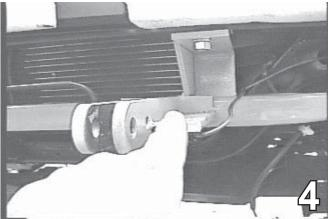
Hold the baseplate up so it straddles the frame and the front braces lay flush to the bottom of the metal bumper and the center brace lines up to an existing hole in the lower cross member.
