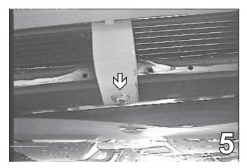
Use the 3/8" -16 x 1 1/4" hex bolts and 3/8" whiz nut with 14" wire for the lower brace, tighten the nut and the bolt. Use LOCTITE red with each bolt throughout the installation.
