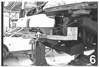
Clamp the baseplate so the two braces are flush with the bottom of the metal bumper. Drill 3/8" holes and use the 3/8"-16 x 1 1/4" hex bolt, 3/8" lock washer, 3/8-16 hex nut, and the 3/8" flat washer.
