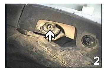
Use the 8MM socket to remove a bolt from inside the front wheel well on the fascia corner. Do this to both sides of the vehicle.
