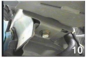
10. Using the baseplate as a template, drill the remaining holes into the frame webbing and radiator support with the 13/32" drill bit. Align the 3/8-16 nut plate on the back side of the radiator support with drill hole. Tighten the 3/8-16 hex bolt and lock washer. Insert the 3/8-16 hex bolts into the drilled holes on the top of the frame webbing and tighten 3/8-16 hex nuts and lock washers. Do this to both sides of the vehicle.
