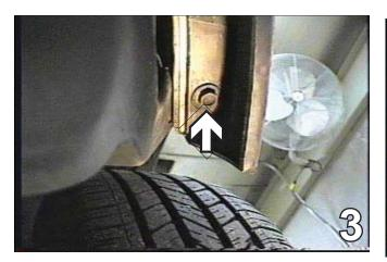
3. Using the 10MM socket, remove two metric bolts from the bottom edge of the fascia corner, just forward of front tire. Do this to both sides of the vehicle. Unplug the fog lights, pull fascia forward. Set it and the bolts aside to be reinstalled later.
