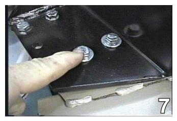
7. Remove the two metric bolts on the top of the metal bumper with the 12MM socket. Do this to both sides of the vehicle. These factory bolts will not be reinstalled. Align and center the baseplate with these bumper holes, tighten the 8MM-1.25 hex bolts, 8MM lock washers provided. Do this to both sides of the vehicle. Do NOT apply LOCTITE Red at this time.
