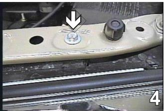
If a right angle drill is available, go to step 7. If not, the head light assemblies need to be removed. Use the 10MM socket to remove two bolts on the top side of head lights. Do this to both sides of the vehicle.
