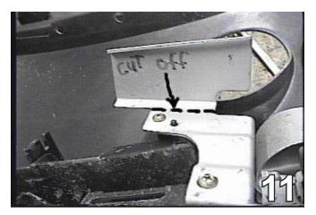
11. Cut off the metal supports on the inside of the fascia. **NOTE:** Cut at location of black line marked on the fascia, as indicated by the dotted line in the photo above.
