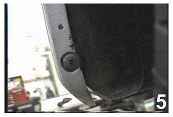
5. Just forward of the front tires is one Phillips screw to be removed. Do this to both sides of the vehicle.
