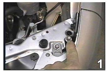
1. With the 10MM socket remove metric bolt on the top edge of the fascia, just above the headlight assemblies. Do this to both sides of the vehicle.
