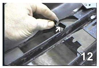
12. Trim off the plastic tabs on the back side of fascia. These are found near the grille opening area that attachment tabs will go through. Do this to both sides of the vehicle.
