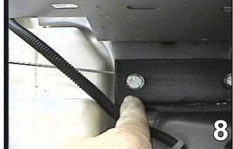
Make sure that the baseplate is centered. Using the baseplate as a template, drill a hole with a 13/32" drill bit into the radiator support using the outermost hole of baseplate. Using the 3/8-16 Whiz Nut, 3/8-16 x 1 1/4" hex bolts, 3/8-16 nutplate 1/4" x 1" x 1", and the 3/8" lock washer. Be sure to use LOCTITE Red on all bolts.
