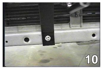
10. Drill all remaining holes and tighten all fasteners. Making sure that LOCTITE Red is used on all bolts. Tighten according to the torque specifications on the front sheet of this document.
