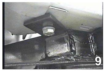
Drill 13/32" holes on the underside of the metal bumper with the 3/8-16 nutplate 1/4 " x 1" x 1', 3/8-16 x 1 1/4" hex bolt, and the 3/8" lock washer. Be sure to use LOCTITE Red on ALL bolts.
