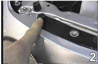
2. Remove the nine Phillips head bolts from the top of the fascia and set black support plate aside to be reinstalled later.
