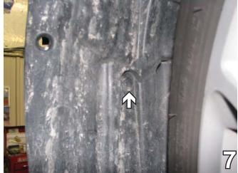
7. On the driver's side only, just forward of the front tire, remove the Christmas tree push pin. Set air baffle and push pin aside to reinstall later.
