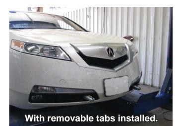
Be sure that ALL electrical connections are plugged in properly and functioning **BEFORE Installing the fascia.**
