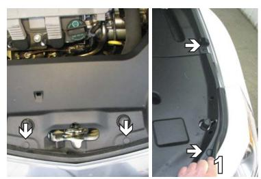
1. Remove six push pins from the plastic above the radiator, three on each side. Remove the plastic from the top of the radiator. Set pushpins aside to reinstall later.
