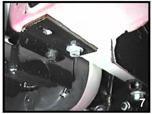
BE SURE TO USE LOCTITE® RED ON ALL BOLTS BEFORE TIGHTENING. TIGHTEN ALL BOLTS ACCORDING TO THE TORQUE CHART ON THE FRONT PAGE OF THESE INSTRUCTIONS OR ON PAGE 3 OF THE BASEPLATE TOWING GENERAL INSTRUCTIONS.
