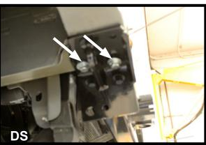
9. Attach baseplate to the underside of the bumper using the existing two (2) holes. Use 3/8"-16 x 2" bolts, 3/8" flat & lock washers and 3/8" nut plates. Use the backing plates on the inside of the frame in between the frame and nut plates.
