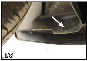
2. Release the push pin that is located on the lower portion of the backside of the fascia, directly in front of the tire, using a flat screwdriver.
