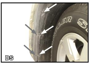
1. Release the three (3) push pins located in the wheel well area of the vehicle using a flat screwdriver. Then remove the two (2) pop rivets.
