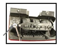
Remove the plastic cap in the tail light assembly and insert 3 wire automotive socket according to the BX8869 installation instructions.
