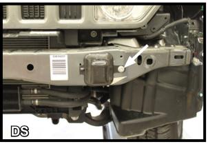
5. Remove cups on the bumper using a 10mm socket. These holes will be used later for nut plate installation for the baseplate.
