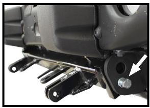
Align the baseplate between the bumper brackets. Insert one (1) of the 1/2"-13 x 1-3/4" hex head bolts and 1/2" lock washers in the bottom hole and tighten securely. Do this on both sides.
