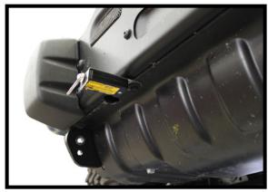
Align the hole of the breakaway switch bracket and use the fasteners provided.
