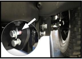
Using a rubber mallet, insert the spacer tube into the top hole until it is flush with the hole. Insert one (1) of the 1/2"-13 x 1-3/4" hex head bolts, 1/2" lock washers and 1/2" flat washers and tighten securely. Do this on both sides.
