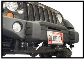
If installing a breakaway switch, use a 13MM socket to remove one (1) of the existing bolts on either side of the bumper.
