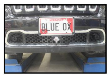
11. Hold the fascia as close to its original position, mark and trim the fascia around the convenience links and attachment tabs. Reinstall the fascia and fascia cover.
