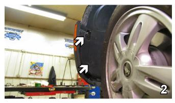
Just forward of front tire, on wheel well, are two phillips head push pins to remove, on both sides.
