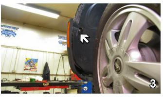
3. Locate opening in wheel well just forward of front tire, remove two metric bolts with the 8MM socket, on both sides.
