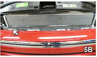
5. Remove three metric bolts from the lower edge of front fascia with the 10MM Socket. Release the four clips on the top edge of fascia, pull fascia forward, unplug all electrical connections and set fascia aside carefully.
