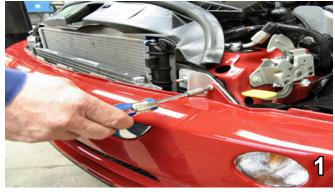
Using the 30 Torx, remove the bolts from the top side of fascia.
