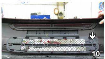
10. Hold fascia as close to its original location as possible on the vehicle. Mark and trim lower grill around the convenience links and attachment tabs. Reinstall fascia. Be sure all electrical components are plugged in properly.
