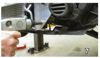
Remove the two metric hex nuts just below metal bumper with the 13MM socket, on both sides.
