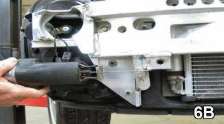
Locate tow plate bracket on passenger's side
