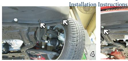
4. Remove the two phillips screws from the lower edge of front fascia, on both sides.
