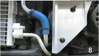
8. Using a utility knife, make a slit the length on blue 3/8" tubing, wrap the tubing onto driver's side upper coolant line as shown. Secure the tubing to the line with zip ties. This will protect coolant line from rubbing against the back of baseplate.
