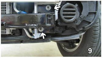
9. Align holes of baseplate with studs just below metal bumper and reinstall four metric hex nuts from step 7 (Driver's side shown in photo above). Be sure and use loctite on all bolts before tightening. Tighten all bolts according to torque chart in the General Instruction sheet.
