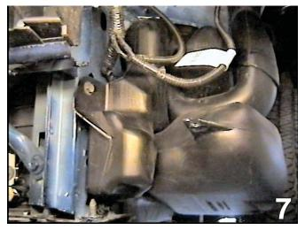
7. Remove the windshield washer reservoir using the 10MM socket on the three side bolts, one bolt on the bottom, with the 7MM socket and one Phillips screw on the outer tubing. Pull the reservoir down, disconnect the electrical connections, cap pump tube and set aside to be reinstalled later. Remove the horn bracket on the passenger's side of the vehicle with the 10MM socket.
