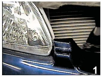
1. Remove four pushpins from the top side of the fascia. Set the pushpins aside to be reinstalled later.
