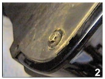
2. Using the 7MM socket, remove three metric bolts inside the wheel well. Do this to both sides of the vehicle.
