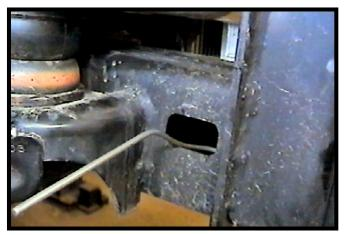
Insert a nut plate into the opening just behind the drilled hole on the outside of the frame to align with the drilled hole. Install a 1/2"-13 x 1-3/4" bolt with lock washer into the bottom hole.
