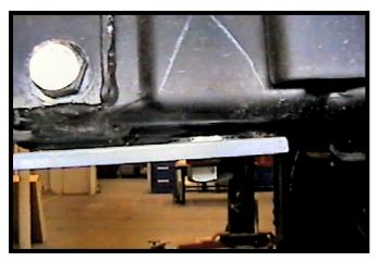
Using the baseplate template, drill the lower hole into the frame with the 17/32" drill bit. Do this to both sides of the vehicle. Loosen bolts installed in Step 9, slide the 1/2" flat washer between the frame and the baseplate to align with the drilled hole.
