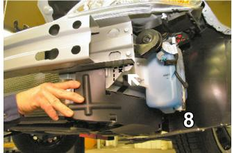
Mark a line from outer edge of bumper brace, along the bottom edge of metal bumper and down, flush with the outside edge of frame rail, both sides (view of driver's side). Remove this area with the reciprocating saw, both sides.
