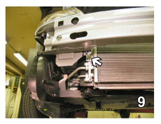
9. Mark a line from inner edge of bumper brace, along the bottom edge of metal bumper and down, flush with the inside edge of frame rail, both sides (view of passenger's side). Remove this area with the reciprocating saw, both sides.
