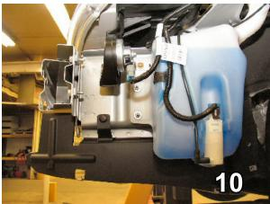
10. Using the 10MM socket, remove the metric bolt from the horn bracket on the driver's side, unplug and set aside.
