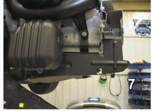
7. Remove the metric bolt from the air dam intake tube on the passenger's side with the 10MM socket.
