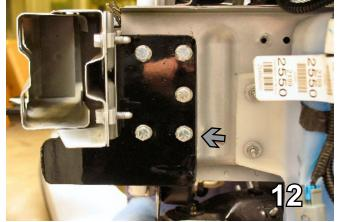
12. Using the baseplate as a template, drill five holes on the driver's side and the four holes on the passenger's side with the 13/32" drill bit. Insert the nut plates into the end of frame rail, just behind metal bumper bracket to align with drilled holes, insert 3/8-16 x 1 1/2" hex bolts, one flat washer (gray arrow) and lock washers into baseplate/ drilled holes with the 9/16" socket, both sides.
