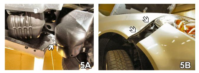
5. Remove the lower metric bolt just forward of the front tire (left photo), on fascia's upper corner, using the 10MM socket, both sides. Loosen the top and bottom remaining metric bolts to release fascia's corner, with the 10MM socket, both sides.
