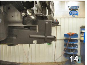
14. Remove existing metric bolt from passenger's side, installed in step 11. Using the 6MM-1.0 x 45MM hex bolt and 1/4" flat washer, reinstall the air intake tube to its original position on the frame.
