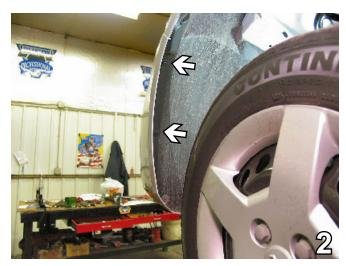
2. Just forward of front tire, on edge of wheel well, are three metric bolts to remove with the 7MM socket, both sides.
