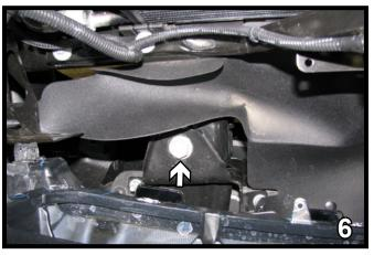
Remove the bolt on top of frame end, just below plastic removed in Step 4 with a 21MM socket. Reinstall the bolt with four (4) 1/2" flat washers. Do this to both sides, one side at a time.
