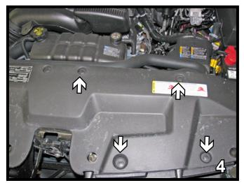
4. Remove four (4) pushpins from the flat plastic piece on top of fascia. Do this to both sides of the vehicle.
