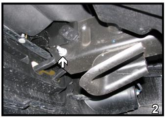
Using a 18MM socket, remove one nut from the outside edge of the frame rail. Pull the tow hook forward and remove it. Do this to both sides of the vehicle. The factory tow hooks will not be reinstalled.
