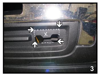
3. Using a utility knife, trim the top part of the tow hook shield. Do this to both sides of the vehicle.
