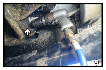
9. Using the existing back hole and the baseplate as a template, drill through to the other side of the frame wall with a 17/32" drill bit. Insert a 1/2"-13 x 5" hex bolt, 1/2" lock washer and 1/2"-13 hex nylon lock nut into the back hole and tighten down. Tighten down both fasteners until the frame squeezes against the baseplate. Do this on both sides of the vehicle.
