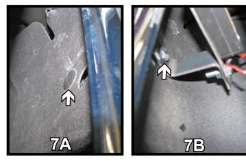
7. Remove two push pins from the opening in the grille (7A). They will be replaced with bolts and brackets (7B). Install the breakaway bracket on the passenger side with 1/4"-20 x 3/4" bolt and 1/4"-20 nut. Attach the breakaway to the bracket also with 1/4"-20 x 3/4" bolt and 1/4"-20 nut.
