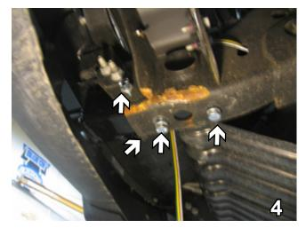
Start all four bolts, remount any hole if necessary as every vehicle is different. Insert 1/2 x 1 1/4" hex bolts with 1/2" lock washers. Be sure to use Loctite Red on all bolts. Do this on both sides.
