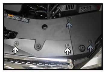
Using a T20 Torx, remove the two (2) screws from the top edge of the fascia (white). Then remove the two (2) push pins (gray). Do this on both sides of the vehicle.
