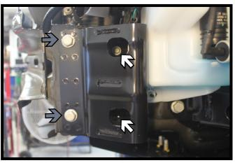
6. **2014 Models Only:** On the driver side, using a 10MM socket, remove the two (2) interior bolts (white) from the reinforcement. Using a 15MM socket, remove the two (2) outer bolts (gray). The reinforcement will not be reinstalled.
