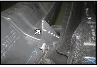
17. **2010-13 Equinox:** Trim the ends of the opening approximately 1" down on the bottom then tapered back to top.
