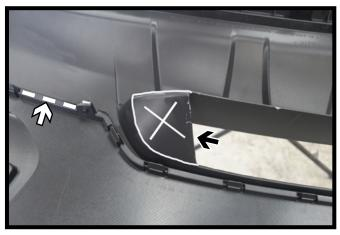
17. **2014 Equinox:** Trim off the end of the styrofoam support above the opening (left). On the end of the opening, trim along the seam as shown (right-black). Then as needed trim off the material between the tabs as needed to clear the baseplate (right-white).
