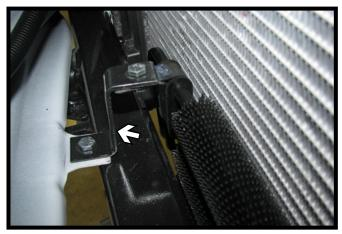
18. If equipped, reinstall the cooler to the existing tabs with the supplied brackets and 1/4" hardware in between the baseplate and radiator.
