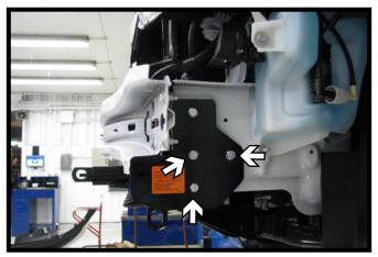
13. Using a 13/32" drill bit, drill the remaining holes thru the frame. Install 3/8"-16 x 2" bolts with 3/8" lock washers into the holes and install 3/8" nut plates inside of the frame. Do this on both sides of the vehicle. Fully tighten all hardware.
