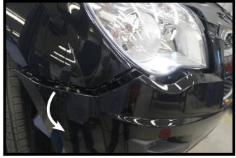
4. Pry the corners of the fascia away from the vehicle. Disconnect all electrical connections and pull the fascia from the vehicle.
