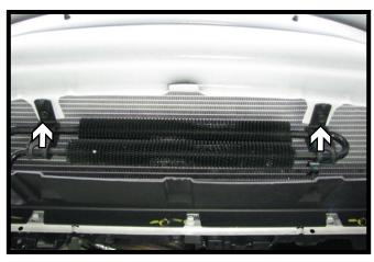
9. If equipped, remove the two (2) bolts from the cooler and move it down to allow the baseplate to be installed.
