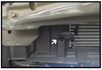
10. Unsnap the temperature sensor and move it aside for baseplate installation.
