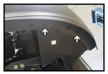
Using a 7MM socket, remove the four (4) screws from the underside of the fascia. There are two (2) on each side.
