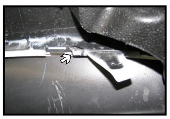
17. **GMC Terrain:** Trim off the corner next to the flap to allow for baseplate clearance. Do this on both sides of the fascia.
