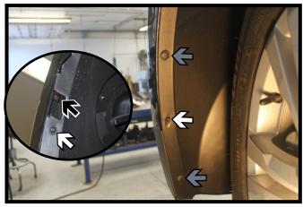
2. **All Models:** Using a T20 Torx, remove the two (2) screws from edge of the wheel well (white). Then remove the two (2) push pins (gray).
