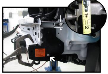
12. Slide the baseplate onto the frame until it is 1-1/8" from the baseplate to the top of the frame (inset). Level and clamp the baseplate securely. Using a 13/32" drill bit, drill a the bottom in the baseplate thru the frame. Install a 3/8"-16 x 1-1/2" bolt into the hole and install a 3/8" lock washer and lock nut on the inside of the frame. Do this on both sides of the vehicle. Recheck the baseplate is level and fully tighten all hardware.
