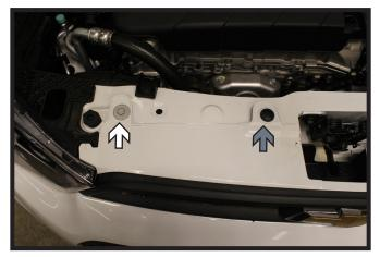
Using a 10MM socket, remove the screw from the top edge of the fascia (white). Then remove the push pin inwards toward the hood latch (gray). Do this on both sides of the vehicle.
