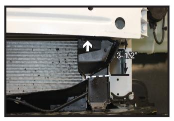
6. Measure down approximately 3-1/2" and cut thru the plastic shielding. Remove the upper push pin and discard the upper portion of the shielding. Do this on both sides of the vehicle.
