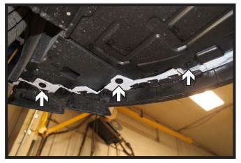
Using a 7MM socket, remove the eight (4) screws from the underside of the fascia. There are three (3) on each side and two (2) in the center.
