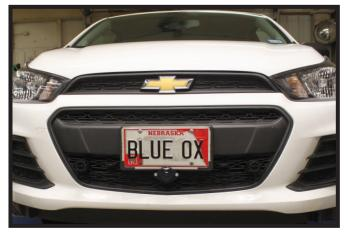
13. Hold the fascia as close to its original position, mark and trim the fascia around the convenience links and attachment tabs. Reinstall the bumper and fascia.
