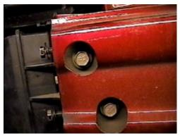
7. Remove four metric bolts from metal bumper front openings using the 13MM socket, disconnect wiring harness and set metal bumper aside. Metal bumper will not be reinstalled.
