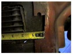
8. Using the reciprocating saw, measure and mark from the top side of lower radiator tray up 2 3/4" and 5" on lower frame, both sides. Then make two 1" horizontal cuts on lower frame bend section back out of the way or cut off.
