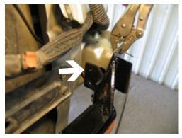
11. In the center bottom hole, use a 3/8 x 1 1/2" bolt. Add a bracket to the back of the baseplate. Align bottom hole of bracket with bottom hole and attach 3/8" lock washer with 3/8" nut plate. Do this on both sides.
