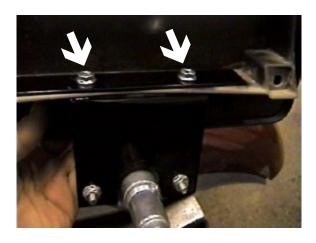
15. Reinstall front fascia and remove license plate bracket using the 10MM socket. Using item 8 as a template, center and drill two holes into the bottom of license plate bracket with the 9/32" drill bit. Install items 8, 10, 11, 12 and 13 to license plate bracket according to drawing on last page. Reinstall license plate bracket.
