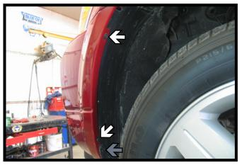
Using a 7MM socket, remove the two (2) screws from the wheel well (white). Then the push pin on the lower corner (gray). Do this on both sides of the vehicle.
