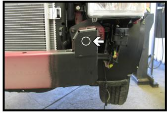
13. Using a 1-1/4" holesaw, drill an access hole on the face of the frame above the bumper. Do this on both sides of the vehicle.
