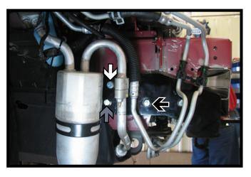
16. On the passenger side, using a 13/32" drill bit, drill the remaining three (3) holes thru the frame. On the lower middle hole, install a 3/8"-16 x 1" bolt with 3/8" lock washer and 3/8"-16" nut (black). Install a 3/8"-16 x 1-1/2" bolt with 3/8" lock washer and 3/8"-16 nut plate into the upper rear hole (white). Install a 3/8"-16 x 1-3/4" bolt with 3/8" lock washer and 3/8"-16 nut plate (gray), using the access hole in front for the nut plates. Tighten all fasteners.
