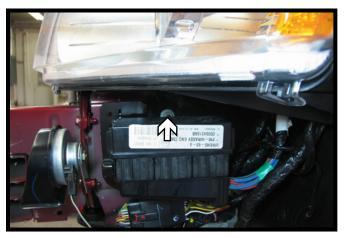
On the driver side, using a 13MM socket, remove the bolt from the wiring harness.
