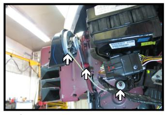
On the driver side, disconnect the horn wire (left). Using a 10MM socket, remove the bolt from the horn bracket (middle). Then using a 13MM socket, remove the bolt from the wiring harness (right).
