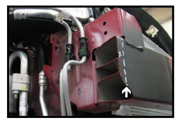
Using a reciprocating saw, trim the end of the bumper off so that it is flush with the frame.
