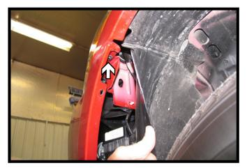
Behind the wheel well cover, using a 7MM socket, remove the screws from the top edge of the fascia. Do this on both sides of the vehicle.
