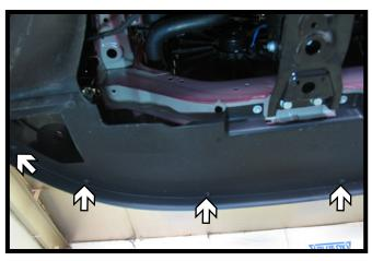
5. Remove the four (4) push pins from the underside edge of the fascia. Do this on both sides of the vehicle. Remove the fascia from the vehicle.
