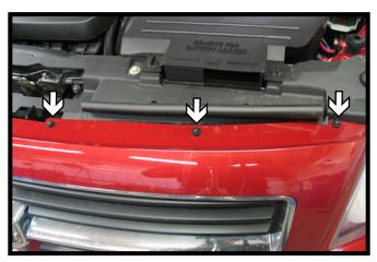
1. Using a T30 Torx, remove the three (3) screws from the top edge of the fascia. Do this on both sides of the vehicle.
