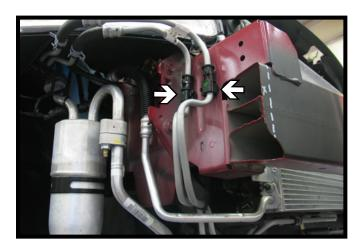
On the passenger side, pry the coolant line clips away from the frame to allow clearance for cutting.
