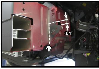
12. Using a reciprocating saw, trim the web 3/4" up from the tab back to the frame. Then down flush with the frame. Do this on both sides of the vehicle.
