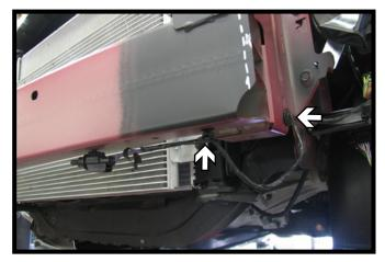
On the driver side, disconnect the sensor wire from the side of the frame and bottom of the bumper to allow clearance for cutting.
