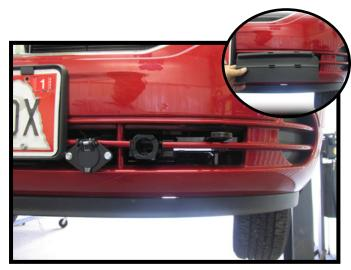
19. Reinstall the wiring harness bolts and horn. On the backside of the fascia, remove the platice panels (inset). Hold the fascia as close to its original position, mark and trim around the attachment tabs. Reinstall the fascia.
