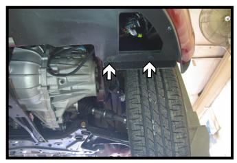
4. Remove the two (2) push pins from the underside corner of the fascia. Do this on both sides of the vehicle.
