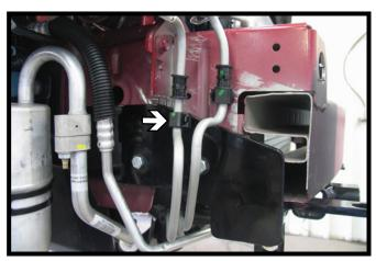
17. On the passenger side, insert the back coolant line clip into the baseplate hole. Insert the front clip back into the existing hole. Reinstall the bolts back into the front brackets of the coolant line.
