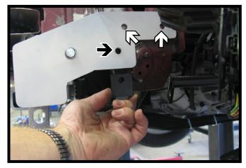
15. On the driver side, using a 13/32" drill bit, drill the remaining three (3) holes thru the frame. On the lower middle hole, insert the spacer in between the frame and baseplate and install a 3/8"-16 x 1-3/4" bolt with 3/8" lock washer and 3/8"-16" nut (black). Install a 3/8"-16 x 1-1/2" bolt with 3/8" lock washer and 3/8" nut plate into each of the rear holes, using the access hole in front for the nut plates. Tighten all fasteners.
