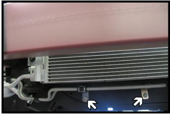
6. Using a 10MM socket, remove the two (2) bolts from the coolant line brackets.
