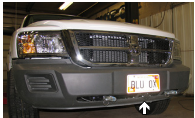
Possible location for the electrical bracket
