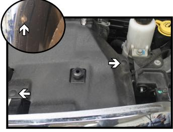
1. **2010-13 Models:** Remove the two (2) pins from the radiator cover. Do this on both sides of the vehicle. Set the cover aside.
