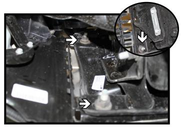
Using a 18MM socket, remove the three (3) nuts from the backside of the bumper. Do this on both sides of the vehicle. Remove the bumper and set aside.
