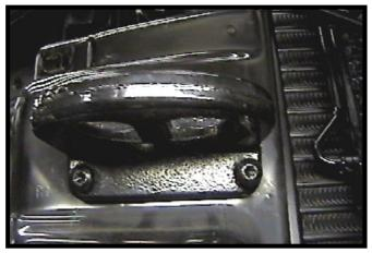
4. Remove the four (4) bolts from the tow hook, using a 50 Torx and/or a 18MM socket. Do this on both sides of the vehicle.
