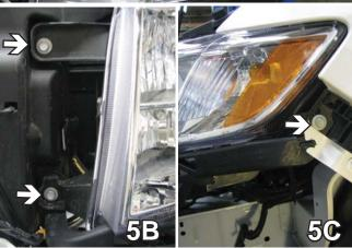
5. Using a 10MM socket, remove four bolts from the headlight assembly. Remove headlight by pulling it forward and disconnecting the electrical connections. Do this to both sides of the vehicle. Set headlight assemblies and bolts aside to be reinstalled later. 6A
