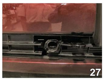
27. Align the fascia to its original position and, using a hack saw blade, trim necessary openings in the grille for the attachment tabs and convenience links.
