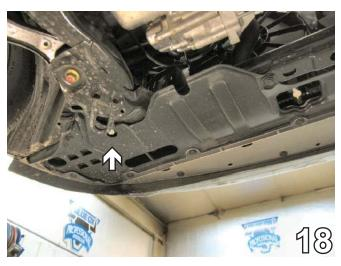
18. Underneath the driver's side, using a 17MM socket, remove the metric bolt from the lower suspension.
