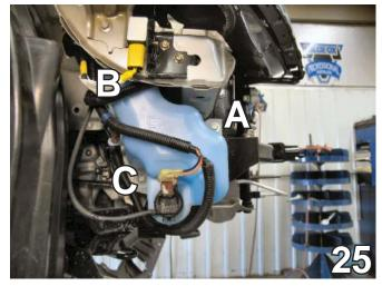
25. Place the windshield washer back to its original position on the passenger's side. Insert the 6MM-1.0 x 30MM hex bolt and fasten with the ¼" flat washer and ¼" lock washer (A in photo above). Insert and tighten original metric bolt removed earlier (hidden behind hoses in photo above - B). Insert 6MM-1.0 x 45MM hex bolt and fasten with the ¼" flat washer and ¼" lock washer using the 3/8" pipe spacer between the washer reservoir and the existing location on the frame. (C in photo above).
