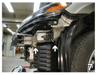
On the driver's side, use a 10MM socket to remove two metric bolts securing the air baffle. Pull down to remove. Set bolts and air baffle aside to be reinstalled later.
