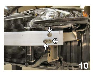
10. Using a 12MM socket, remove three metric bolts from the metal bumper. Do this to both sides of the vehicle. Pull the metal bumper forward. Set metal bumper and bolts aside to be reinstalled later.
