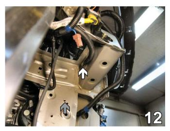
12. On the passenger's side, use a 10MM socket to remove a ground wire from the frame rail. Relocate the ground wire to the rear of the frame extension. The grey arrow is the existing location of the bolt, the white arrow shows where it will be relocated.
