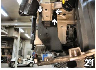
21. Using the support plate as a template, drill three holes into the frame rail with a 13/32" drill bit. Do this to both sides of the vehicle.
