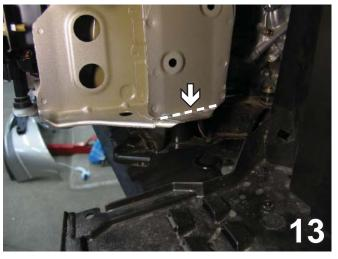
13. Using a reciprocating saw, cut the lip found at the bottom of the radiator support (dotted lines in graphic) to gain access to the area beneath it. Do this to both sides of the vehicle.
