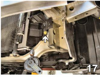
17. Using the 12MM socket, remove the metric bolt from the lower part of the horn shield. Set shield aside. It will not be reinstalled.
