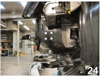
24. Slide the baseplate endplate to the outside of the support plate and align with the existing four holes of the support plate. Ensure baseplate is level with the vehicle and tighten all bolts.
