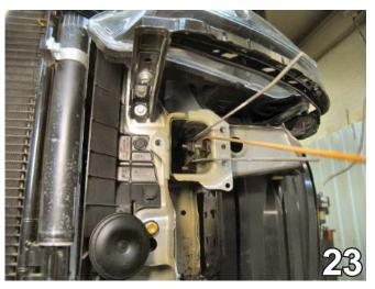
23. Insert 3/8-16 nut plates through the frame rail opening and align with the three drilled holes. Insert 3/8-16 x 1 ½" hex bolts and 3/8" lock washers and tighten. Do this to both sides of the vehicle.
