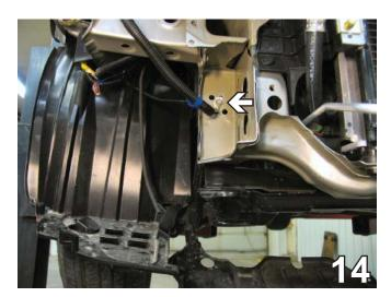
14. Using a 10MM socket, remove a ground wire from the forward facing section of the radiator support on the passenger's side.
