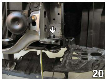
20. Align support plate so ½-13 x 1 ¼" hex bolt can be inserted into the support plate and through the bottom of the radiator support. Tighten with ½" flat washer, ½" lock washer, and ½-13 hex nut. Finish tightening the metric bolt under the lower suspension.
