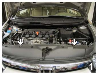
1. Remove two push pins from the top of the fascia. Set push pins aside to be reinstalled later.
