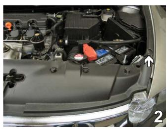
2. To the rear of the driving light, remove a Christmas tree pushpin. Set pushpin aside to be reinstalled later. Do this to both sides of the vehicle.
