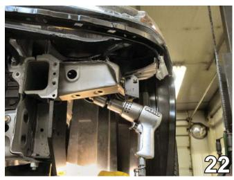
22. The upper-most hole in previous step requires drilling at an approximate 45 degree angle.
