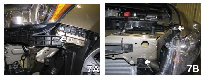
7. Remove the headlight by removing the three bolts around it and unplug the electrical connections. Do this on both sides. Set the bolts and headlights aside to be reinstalled later.
