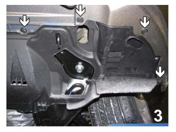
3. Underneath the fascia, remove ten push pins all the way around. Set push pins aside to be reinstalled later.
