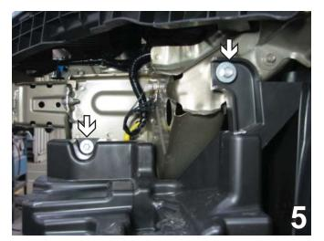
6. On the driver's side, use a 10MM socket to remove the two bolts holding the air baffle. Don't remove the air baffle just pull it back out of the way. Set the bolts aside to be reinstalled later.
