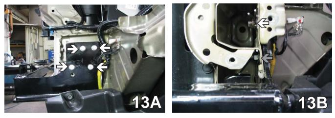
10. Use 3/8-16 x 1 1/4" bolts and 3/8" lock washers in all the holes. The top two attach to 3/8-16 nut plates (13B white arrow) inserted inside the frame. The bottom two attach to 3/8-16 whiz nuts. Be sure to use Loctite Red on all the bolts. Do this on both sides.
