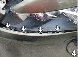
4. Pull the fascia out up to the blinker. Use a small flat screw driver to pry down on each clip in the series of four in order to release the fascia. Pull the two eyelets up off the pins. Do this on both sides. Slide the fascia off, disconnect fog lights and set aside carefully to be reinstalled later.
