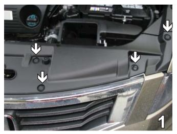
Remove eight push pins in order to remove the radiator cover. Do this to both sides of the vehicle. Set cover and push pins aside to be reinstalled later.
