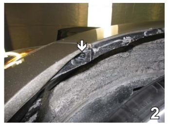
2. In the corner of the fascia, remove the Phillips screw. Do this to both sides of the vehicle. Set screw aside to be reinstalled later.
