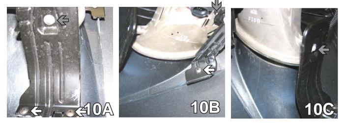
10. Using the Phillips screw driver, remove the three Phillips screws to take the fog light bracket off the back of the fascia (white arrows). Continue to remove three additional screws to take the bulb housing off. Do this on both sides. Set the screws aside to be reinstalled shortly.
