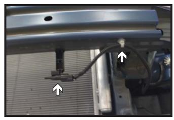
Disconnect the temperature sensor from the underside of the bumper and set aside.
