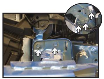
7. Using a 12MM socket, remove the five (5) bolts on both sides of the bumper and set it aside.
