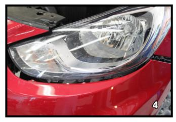
4. To remove fascia, lift up and pull out between the front tire and headlight as shown in the above pictures. Do this to both sides.
