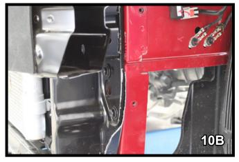
10. With reciprocating saw, cut lower bumper guard (flush with metal brace) where indicated on 10A. Do this to both sides. An example of the completed trimming is referenced in 10B. Reinstall bumper using existing bolts.
