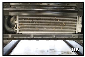
11. On passenger's side only, with utility knife, cut plastic guard even with bottom of metal bumper and remove it from the front of the vehicle (11A). The plastic guard will not be reinstalled. Front view of how the grille looks after plastic guard is removed is shown in 11B.
