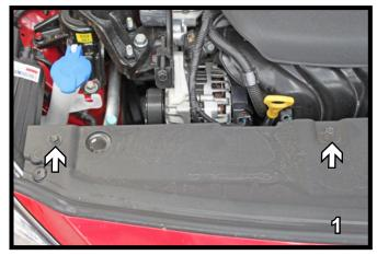
1. To remove the radiator cover, use a 10MM socket, remove four (4) bolts (white arrows - 2 per side). Then remove the two (2) push pins on the drivers side (gray arrows).
