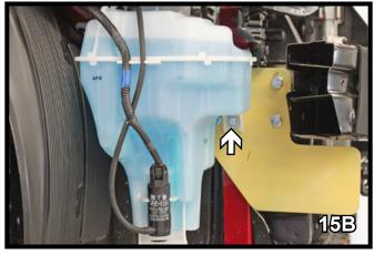
15. Reinstall washer reservoir on passenger's side using existing bolts in the back of the reservoir (15A) and on the side of the reservoir, use 6MM-1.00 30MM hex bolt into existing hole with 3/8" flat washer and 3/8" lock washer (15B). Reattach fluid lines and electrical connections.
