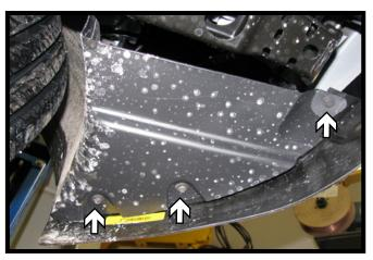
5. Underneath the fascia in the corner in front of the tire, using an 8MM socket remove three (3) screws. Do this on both sides of the vehicle.
