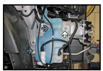
7. Using an 8MM socket, remove the bolt on the top (white). Using an 11MM socket, remove the two (2) bolts on the sides (gray). Remove the windshield washer reservoir, disconnect the two hoses and plug them.
