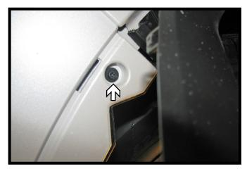
4. Just forward of the front tire on the fascia's corner pry loose the protective rubber edging, remove the screw with a Phillips screwdriver or 5.5MM socket. Do this on both sides of the vehicle.
