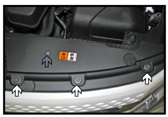
Using a 10MM socket, remove three (3) screws (white arrows) from the plastic cover on the top side of the fascia. Also remove the push pin (gray arrow). Do this to both sides of the vehicle. On the passenger side, there will be four (4) screws to remove.
