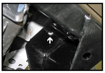
13. Using the baseplate as a template, drill a hole underneath with a 17/32" drill bit. Install a 1/2"-13 x 1-1/2" bolt and 1/2" lock washer with 1/2" wire nut. Do this on both sides of the vehicle.
