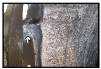
Just forward of the front tire pull the cover back, remove the screw. Do this to both sides of the vehicle.
