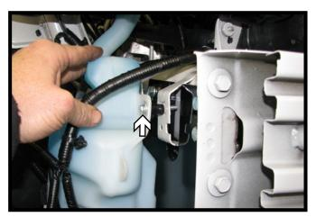
15. Reattach the windshield washer reservoir, using a 6MM-1.0 x 45MM bolt on the top front hole with 3/4" spacer tubes on all three (3) bolts.
