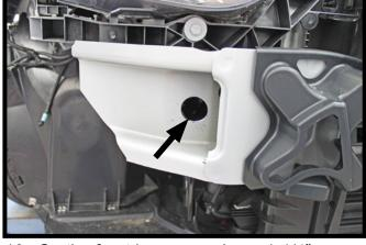
10. On the front bumper, using a 1-1/4" hole saw, slowly drill a hole centered vertically and horizontally on the flat area as shown. Do this on both sides of the vehicle. NOTE: The hole cut is used to place nut plates for future steps and if available the use of a carbide-tipped holesaw is recommended.
