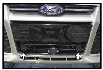
23. Align the fascia as close to its original position and trim the opening for the attachment tabs with a utility knife.
