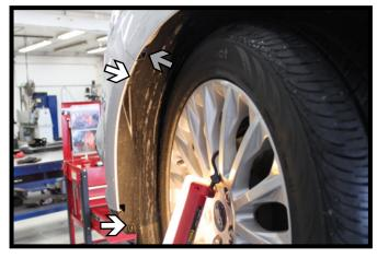
Using a T27 Torx, remove the two (2) screws from the driver's side front wheel well (white arrows). Remove the push pin from the driver's side front wheel well (gray arrow). Repeat this on the passenger's side.
