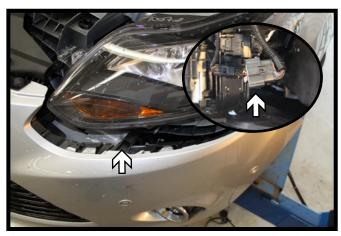
On the driver's side, locate the running lights main electrical cord and disconnect. Under both headlights release the tabs from the body and carefully remove the fascia.
