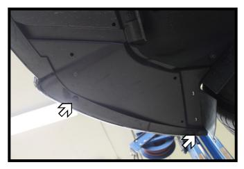
On the underside of the fascia remove the two (2) pushpins from the outer edge. Repeat this on the other side of the vehicle.
