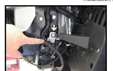
20. Bend the bracket back to it's original location and reinstall the existing bolt.
