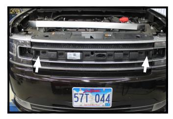
2. Remove the two (2) 10MM screws from face of the grille. Remove the grille from vehicle and set aside for later installation.
