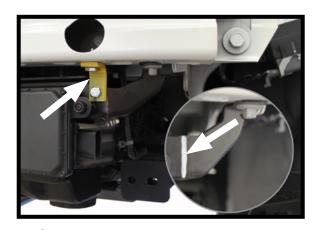
7. On the driver side, install the support bracket onto the bumper and ACC sensor bracket as shown. Mark and drill the holes with a 1/4" drill bit. Attach the bracket with 1/4"-20 x 3/4" bolts and 1/4"-20 lock nuts.
