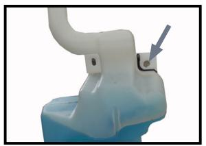
14. Prior to reinstalling the windshield washer fluid reservoir, notch the reservoir as shown.
