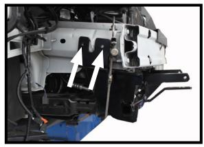
11. Securely clamp the baseplate onto the vehicle's bumper. Make sure the baseplate is level. Then use the baseplate as a template and drill the sides holes with a 13/32" drill bit. Install the 3/8"-16 x 1" hex head bolts, 3/8" lock washers and 3/8"-16 nut plates. Do this on both sides of the vehicle.
