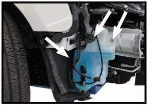
6. On the passenger's side, remove the windshield washer fluid reservoir using a 10MM socket to remove three (3) bolts. There are two (2) on the front of the reservoir and one (1) towards the back.
