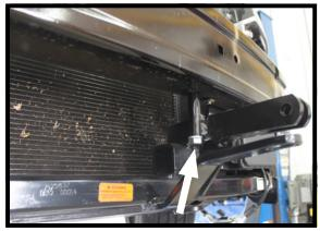
12. Drill a hole thru the bumper with a 17/32" drill bit, using the tube as a guide. Install a 1/2"-13 x 4-1/2" bolt, 1/2" lock and flat washer, with a 1/2" nut plate inside the bumper. Do this on both sides of the vehicle.
