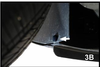
3. Remove the three (3) 5.5MM screws from the wheel well. (3A) Remove the push pin located on the inside corner of the wheel well. (3B) Repeat on other side of vehicle.
