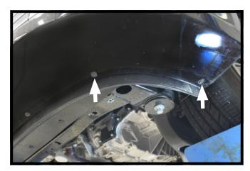
4. Remove the eight (8) 5.5MM screws from underside of the fascia. Remove the fascia from vehicle and set aside for later installation.
