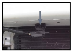
10. Reclip the air temperature sensor to the bumper.
