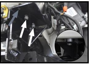
13. Drill the bottom holes using a 13/32" drill bit. The outer most hole requires six (6) 3/8" flat washers for spacers (gray). Do this on both sides of the vehicle.
