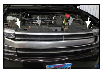
Remove the two (2) 10MM (white) and two (2) phillips head (gray) screws from the top of the grille. Then using a straight screwdriver pop out the chrome trim insert from the grille.
