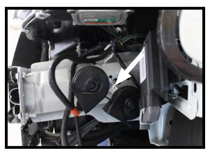
5. On the driver's side, use an 8MM socket to remove the horn bolt bracket. Bend it slightly over to the side temporarily.
