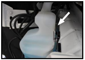
15. Reconnect the windshield wiper fluid reservoir using the existing fasteners. Use the seven (7) 1/4" flat washers that were provided as spacers on the innermost hole.
