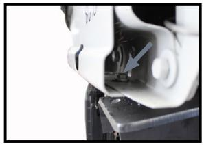
Using a hammer and flat screwdriver, remove the nut on the inside of the bumper on the driver's side.
