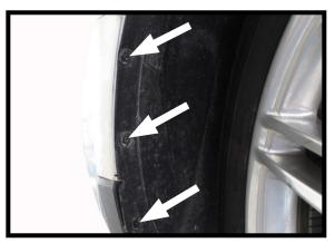
Remove the three (3) bolts that are located just forward of the front tire using a 5.5MM socket. Do this on sides of the vehicle.
