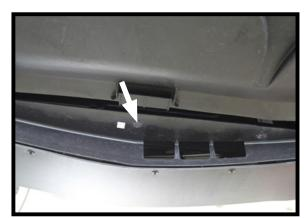
3. There are three (3) large push pins located on the underside of the vehicle. Use a flat screwdriver to remove them.
