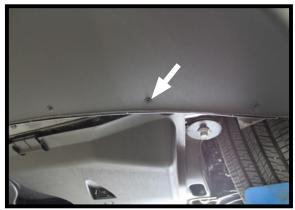
4. Using a 5.5MM socket, remove the seven (7) bolts that are located on the underside towards the front of the vehicle.
