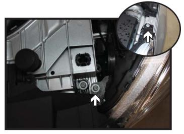
Using a T30 Torx, remove the two (2) screws from the headlight, disconnect and set aside. Do this on both sides of the vehicle.
