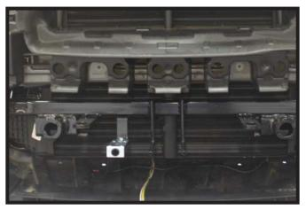
18. **Optional Breakaway (Baseplates with Serial# lower than 00045)**: Install the bracket to the existing hole in the crossmember (inset) with a 1/4" bolt and lock nut. Install the breakaway to the bracket with the supplied 1/4" hardware (Left).
