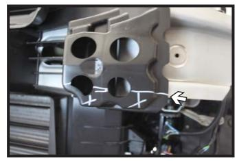
12. Trim the plastic shielding just flush or a little past as shown for baseplate clearance. Do this on both sides of the vehicle.
