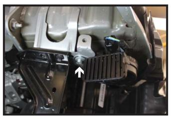
9. Using a 10MM socket, remove the screw from the PS horn and set the horn aside.
