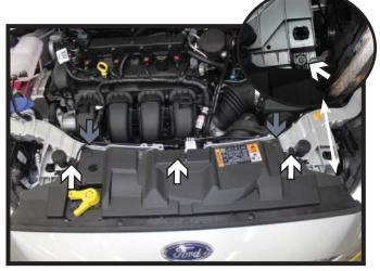
2. Using a T30 Torx, remove the five (5) screws from the top edge of the fascia (white). Remove the two (2) push pins from the outer edges (gray).
