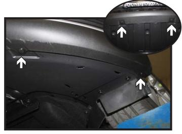
5. Remove the six (6) push pins from the underside of the fascia. There are two (2) in front of each wheel and two (2) in the middle.
