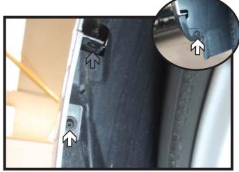
Using a T30 Torx, remove the two (2) screws from the edge of the wheel well (white). Also remove the push pin from the fascia/fender joint (gray). Do this on both sides of the vehicle.
