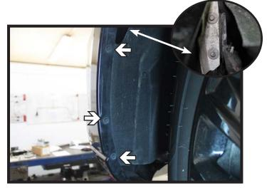
Using a 10MM socket, remove the three
