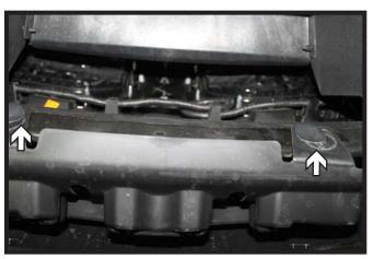
On the underside of the fascia towards the middle, remove the two (2) push pins.
