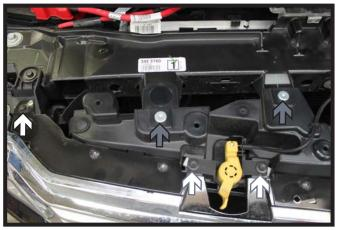
Using a T30 Torx, remove the four (4) screws from the top edge of the grille (gray). There are two (2) on each side.
