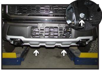
3. Using a 15MM socket remove the six (6) bolts holding the skid plate.
