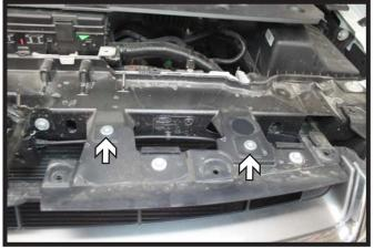
Using a T30 Torx, remove the four (4) screws from the top edge of the grille. There are two (2) on each side.
