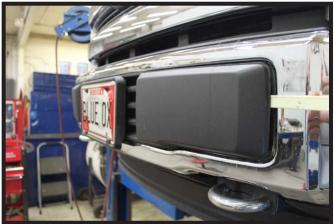
1. Unsnap the plastic cover from the face of the bumper. Do this on both sides of the vehicle.
