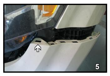
5. The fascia is then ready to be removed from the vehicle by grabbing in front of the tire, lift and pull the fascia ends out to the side to release and then pulling it forward. Use a screwdriver to pop the fascia over the knob at the end (white arrow). Do this to both sides of the vehicle. Set fascia aside carefully.
