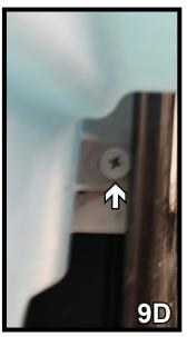
9. On the passenger side, to remove the washer reservoir, remove the plastic push pin on top (9A). Using a 10MM socket, remove the two bolts one above the other (9B & 9C). Remove the screw on the right side to remove the washer reservoir (9D). Disconnect the hoses and wires and plug the hoses.
