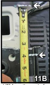
11. Mark straight over 1 1/2" from the end of the frame. Using a reciprocating saw, trim over and straight down 4" flush with the bottom of the frame. Do this to both sides of the vehicle.
