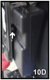
10. On the driver side, using a 8MM socket, remove the air box and shielding. On the underside of the vehicle, remove the three (3) screws from the side of the shield (10A) and the two (2) screws at the front of the shield (10B). After removing the shield remove the one (1) screw from the inside of the frame (10C). On the topside of the air box remove the one (1) screw (10D), then remove the airbox from the vehicle.
