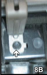
8. If equipped with coolant lines, on the passenger side, using a 10MM socket remove the two bolts supporting the coolant line up. Let the line hang down during the cutting.
