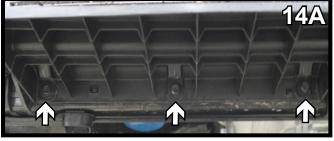
14. On the 2013 Models only, using a 8MM socket, remove the three (3) lower bolts (14A) and the upper bolt (14B) from the lower air baffle. This baffle will not be reinstalled.
