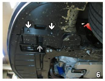
6. Remove two (2) christmas tree pushpins (see white arrows) and one (1) regular pushpin (see grey arrow) from the lower corner of belly pan. Do this to both sides of the vehicle. Set pushpins aside to be reinstalled later.
