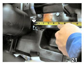
21. On the passenger's side upper rear of the air dam, use the utility knife to make a 1" horizontal cut level with the opening next to the air dam then trim vertically to remove this portion of the air dam.
