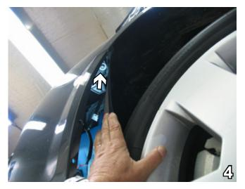
Push wheel well cover aside to remove one metric bolt using the 10MM socket. Do this to both sides of the vehicle. Set bolts aside to be reinstalled later.
