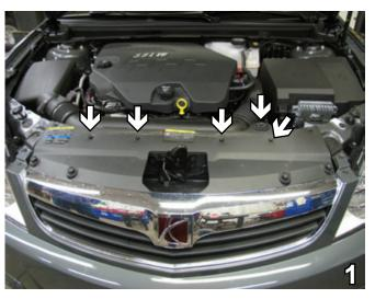
On top of the radiator cover, remove five (5) metric bolts using the 10MM socket. Set bolts aside to be reinstalled later.
