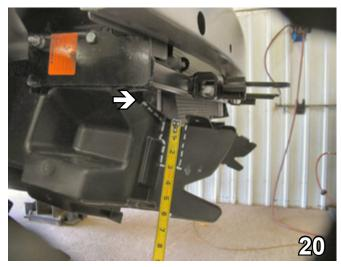
20. Mark the passenger's side of the air dam from the back portion of lip diagonally to the bend and down 3 inches around the contour of the air dam mold. Then mark straight down from the air dam tab three inches and horizontally back to the air dam contour and trim this area with the utility knife.
