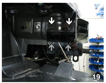
19. On the passenger's side, insert 3/8" nut plates through opening in the bottom of frame rail and align to the upper two (2) holes (see white arrows). Install 3/8"-16 x 1-1/4" hex bolts with 3/8" lock washers and tighten to nut plates. Install 3/8"-16 x 1 1/4" hex bolts with 3/8" lock washers and 3/8"-16 hex nuts to the lower two holes (see grey arrows). Trim excess nut plate wires.
