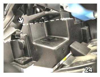
24. On the driver's side, approximately 1" from the top of the air dam, cut horizontally from the front of the air dam to the back.
