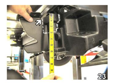
23. On the driver's side, just behind air dam tab, cut down 3". Then, cut horizontally toward rear of air dam approximately 2". Cut upwards to the top, following the contour of the air dam.
