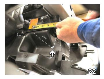
22. On the passenger's side of the air dam, just behind the tab, mark 3" down and 2" horizontally. Then mark upwards, following the contour of the air dam, to the top of the air dam and trim away this area with the utility knife.
