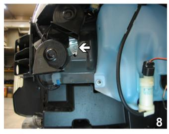
On the driver's side, disconnect electrical from the horn. Using the 10MM socket, remove one (1) metric bolt from the horn bracket. Set bolt and horn bracket aside to be reinstalled later.
