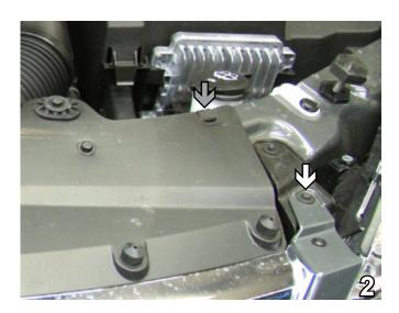
2. Using the 7MM socket, remove one (1) metric bolt from the top corner of fascia (see white arrow). On the top corner of radiator cover, remove one (1) clip (see grey arrow) using the flat screwdriver. Do this to both sides of the vehicle. Pull radiator cover forward to remove. Set bolts, clips and radiator cover aside to be reinstalled later.
