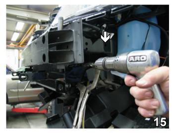
15. On the driver's side, align the upper back hole of the baseplate with the existing horn bracket hole and clamp in place with the vise grips. Using the baseplate as a template, drill the three (3) remaining holes into the frame using the 13/32" drill bit.
