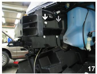
17. On the driver's side, insert 3/8" nut plate through opening in the bottom of the frame rail and align to the upper front hole (see white arrow). Install 3/8"-16 x 1-1/4" hex bolt with 3/8" lock washers and tighten to nut plate. Reinstall horn bracket to upper back hole using 6MM hex bolt, 1/4" lock washer and 1/4" flat washer (see grey arrow). Trim excess nut plate wire.
