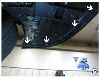
Using the 7MM socket, remove four (4) metric bolts from inside front edge of fascia. Do this to both sides of the vehicle. Pull fascia forward to remove. Set bolts and fascia aside to be reinstalled later.
