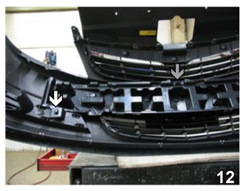
12. Lay fascia face down on a smooth, flat surface. Press in to release clip on the side of fascia support (see white arrow). Do this to both sides of fascia support. Press back to release clip on center of fascia support (see grey arrow). Pull fascia support to remove.
