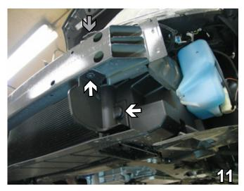
11. Remove one (1) pushpin from the air dam and one (1) from the bottom of metal bumper (see white arrows). Remove one (1) pushpin from top of metal bumper (see grey arrow). Pull air dam forward to remove. Do this to both sides of the vehicle. Set pushpins and air dams aside to be reinstalled later.
