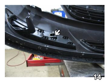
14. Using the utility knife, remove the tab from the back corner of the fascia. Do this to both sides of vehicle.
