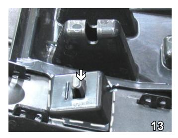
After removing fascia support, use the utility knife to remove the clip on both corners of fascia support.
