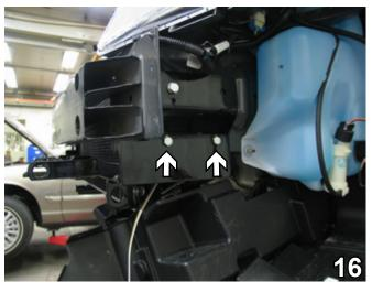
16. Install 3/8"-16 x 1-1/4" hex bolts with 3/8" lock washers and 3/8"-16 hex nuts to lower two (2) holes.
