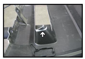
Hold the fascia as close to it's original position and mark the backside of the fascia, trim as needed. Reinstall the fascia.
