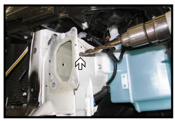
10. Using a 17/32" drill bit, ream out the existing hole in the frame as shown. Do this on both sides of the vehicle.
