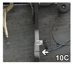
10. Move the bracket out of the way by sliding it up. Measure 7" up. Reroute the wire up and reattach the bracket so that the bottom of it is 7" up.
