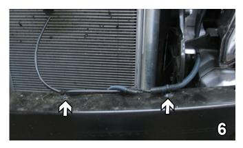
6. Remove the styrofoam. On the driver's side only, using a flat screw driver release the tabs from the top of the bumper and tie the wire loom up in the open area during baseplate installation.
