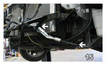
15. Attach baseplate safety cables as in above photos or as close to as possible. If you are unable to place safety cables in this location, position the cables around a solid piece of the frame. Do this on both sides.
