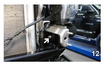
12. Insert 3/8-16 x 1 1/4" hex bolts with 3/8" lock washers attached to 3/8-16 nut plates with inserted into the frame rail on both sides to hold the baseplate in place.
