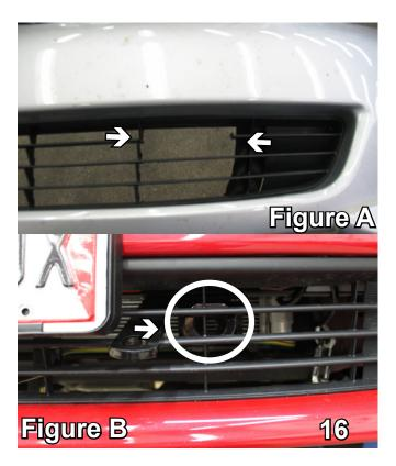
16. Hold the fascia as close to its original position as possible, mark and trim the grill with a utility knife to allow the baseplate receivers to come through. Reinstall the fascia.
