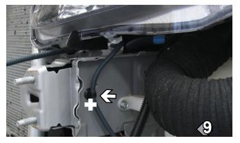
9. On the driver's side pull the wiring out of the existing hole. Drill a hole in the frame rail under but connected with the existing hole using the 1 1/4" hole saw on both sides. This hole will allow the installer to insert the nut plates inside of the frame rail.
