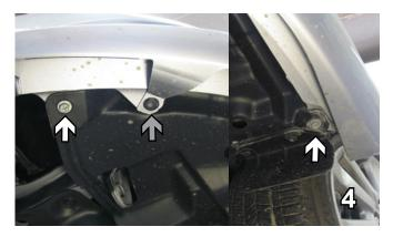
4. Just forward of the front tire underneath, using a 10MM socket, remove the two metric bolts (white arrows). Using a flat screw driver, remove the push pin (gray arrow). Do this on both sides and set aside for later reinstallation.
