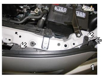
1. Using the Phillips screw driver, remove the Phillips screws (white arrow) from the top corner edge of the fascia. Remove push pin (gray arrow), do this to both sides and set aside for later reinstallation.
