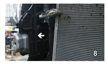
8. Remove the black shield on both sides. It will not be reinstalled.
