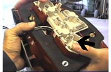
Note: If using the Bx8869,remove electronic circuit board off the back of light assembly, photo to the left shows socket location.
