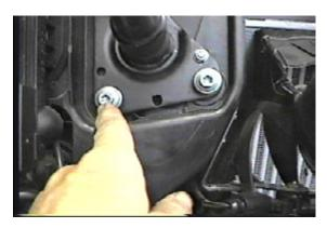
**9.** There are three torx bolts to remove from bumper mounts with the T-45 Torx, each side.
