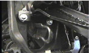
10. Hold baseplate into place, while allowing air dam to fold out of the way, and hand tighten items 2, 3, and 4 on driver's side, then passenger's side. Tighten all bolts. Reference drawing on last page for correct locations of parts (note flat washers on passenger's side). Be sure and use loctite on all bolts before tightening.
