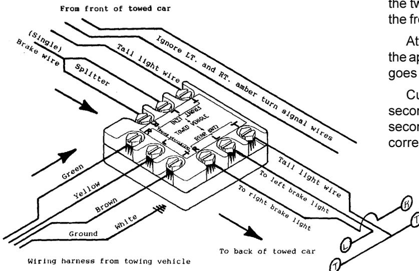
Cut the main brake wire coming from the front, and strip it back approximately 1/4". Use the butt connector provided to connect the stripped wire and the single wire on the splitter, crimp with a wire terminal crimper. Attach the two ends of the splitter to the left and right screws on the front of the connector.
