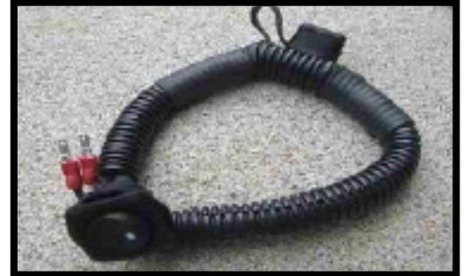
1. Install the two (2) small wire pins into the fuse panel location from where you removed the fuse in the "towed". Press in on the pins until fully seated.
