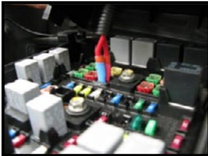
under hood fuse box. Remove the large plastic fuse box cover and remove the high amperage (e.g. 50 amp) fuse. Confirm that the colored connectors on the Fuse ByPass Switch wire (or adapter if supplied) match the pin sizes in the fuse box location from where you removed the fuse. If your manual requires that you remove another mini fuse, typically the 15 amp ECM fuse, you will need an additional mini version of the Fuse ByPass Switch.
