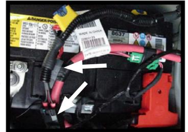
11. Install the fuses into the appropriate fuse holders on the Fuse ByPass Switch harness.
