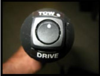
With the car engine and key turned fully off, flip the Fuse ByPass Switch to the **tow** position.
