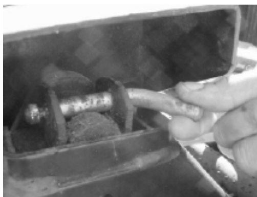
Figure 4 – Removing Hitch Head Right Pin
