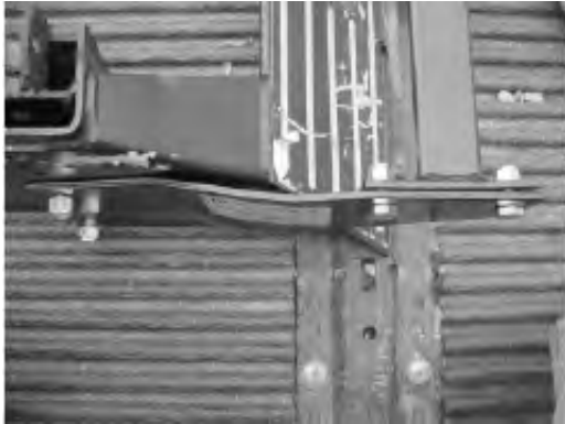
Figure 7 – Crosstube Attachment, Left
