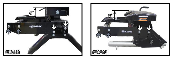
Install the side plates onto the hitch, using two (2) 1/2"-13 x 1-1/4" bolts and 1/2"-13 lock nuts per side and tighten down (white). Install the x-tube in between the side plates, using two (2) 1/2"-13 x 1-1/4" bolts and 1/2"-13 lock nuts per side and tighten down (gray).
