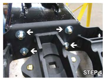
4. Bolt the bracket to the fifth wheel hitch, insert  $1/2-13 \times 1 \ 1/4$ " hex bolts, Grade 8, with flat washers and nylon insert lock nuts. Use a 3/4" socket with ratchet and a 3/4" open end wrench. Torque the bolts to 119 ft lbs.
