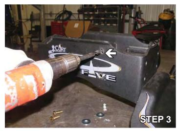
3. Remove the bracket from the fifth wheel hitch. Using a .531 drill bit, drill all four holes. Note: (It is recommended to take the fifth wheel head off before drilling.)
