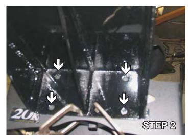
2. Using the BedSaver as a template, mark the holes with a transfer punch.
