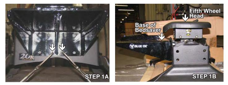
1. C-clamp the bracket of the BedSaver so that the BedSaver is centered from side to side. The dimension from the top of the fifth wheel head to the base of the BedSaver bracket is 5 inches.
