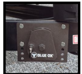
**Bolt Around Method:** Install the appropriate bolts into the top holes of the latch plate and the closest lower holes to the bottom of the frame. Install the backing plates and 1/2"-13 lock nuts on the inside of the frame. Torque to 78 ft/lbs.
