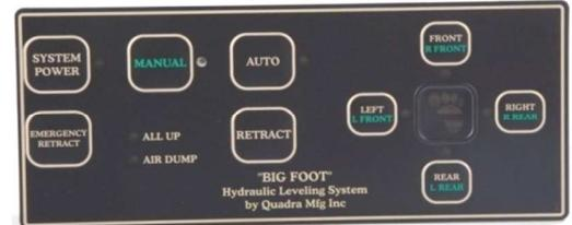
1. Turn panel/system on and let system run through its diagnostic mode. Lights will flash clockwise around the green foot. (System will not operate with the ignition key ON)
