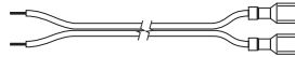
Cables with Quick Disconnects for Motor Cables with Quick Disconnects Only TravelR061b
