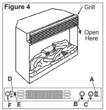
To access the manual controls, open the upper grill by pulling, near the top right hand side, forward and down (Figure 4).
