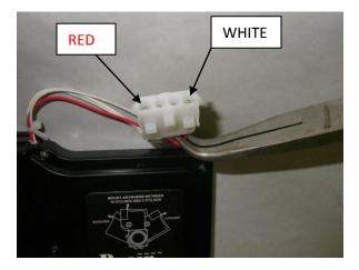
Using a 12vdc battery or battery charger set on 12vdc, put the White wire on the Positive terminal and the Red wire on the Negative terminal.
