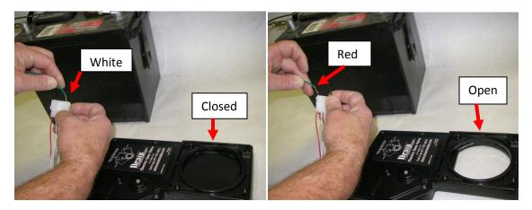
In the event the valve does not OPEN or CLOSE with the above procedure chances are good the valve has failed and needs to be replaced. If the valve works but is very sluggish (opens and closes but very slowly) the valve may need to be removed and cleaned. See Cleaning Procedure.
