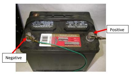
The valve should OPEN in about 1 second! Now reverse the wires by putting the Red wire on the Positive terminal and the White wire on the Negative. The valve should close. If this works do it a few times just to make sure. The problem is in the wiring, the switch, the 12vdc power source, or maybe a blown fuse.
