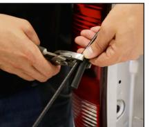
Install the narrow end of the shock on the ball mount.
