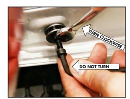
\*WARNING: Over-tightening the nutsert can strip the threads and cause the nutsert to be unusable.
