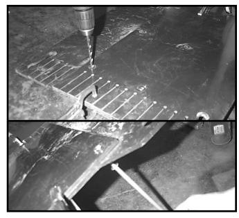
8. Drill six holes through center section with a 9/32" drill bit, (On wider setting, it may require three holes) using existing holes as a template to drill through. Install tee nuts and truss head bolts in these holes and remove clamps. Apply thread lock to the threads.
