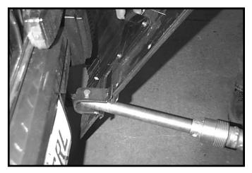
1. Slide right and left wings into Sentry connecting clevis until wings are approximately 1/4" away from bottoming out against clevis.
