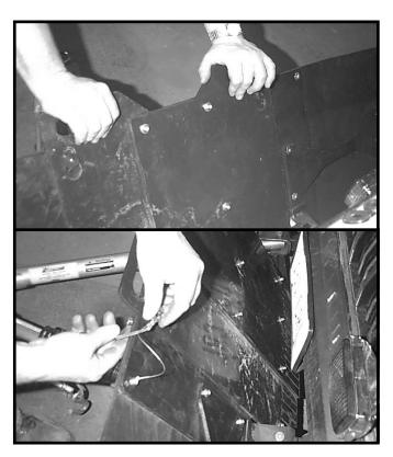
Push down on center section until it snaps into place. Insert pin through hole provided and snap wire over pin to secure Sentry together as a unit. Hole on other side maybe used for a paddle lock for antitheft, if necessary.
