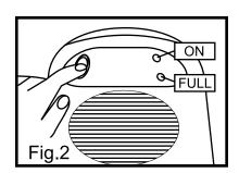
When the water tank is full (Approximately 2 liters). The unit will automatically turn off and the "Yellow" LED (3) will turn on.
