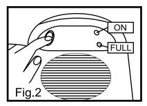
To remove the water tank, first turn the unit off. Then remove the water tank from the unit and empty the water. Place the water tank back into the unit, and turn the unit back on to continue dehumidifying.
