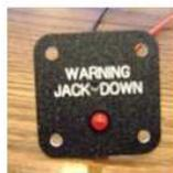
Indicator to be attached to dash in a convenient & highly visible location for the driver to see.
