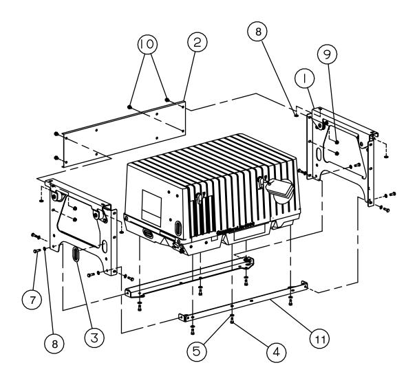
DESCRIPTION SCREW - HHC (3/8 - 16 X 0.75) REF. DESCRIPTION REF. 7. 1. SIDE PANEL ASSEMBLY FLAT WASHER (3/8 HARDENED) 2. **BACK PANEL** 8. NUT - HEX LK (5/16 - 18) **GROMMET** 9 3. SCREW - HHC (5/16 - 18 X 0.75) FLAT WASHER (5/16 - HARDENED) 10. SCREW - HH LK FLG (5/16 - 18 X 0.5 4. 11. RAIL 5.
