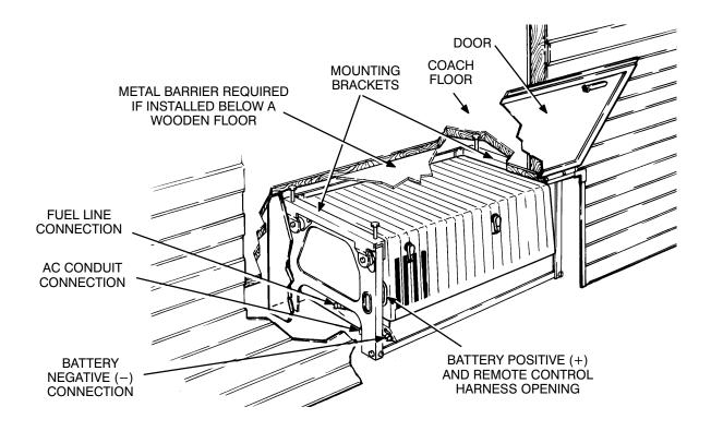
FIGURE 1. TYPICAL UNDER-FLOOR INSTALLATION
